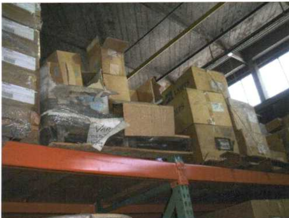
Photo 1 - Unsecured material storage on top rack, Main Storage Area/Supply room
